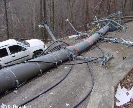
Collapse of pipe poles with bolted flange splices
